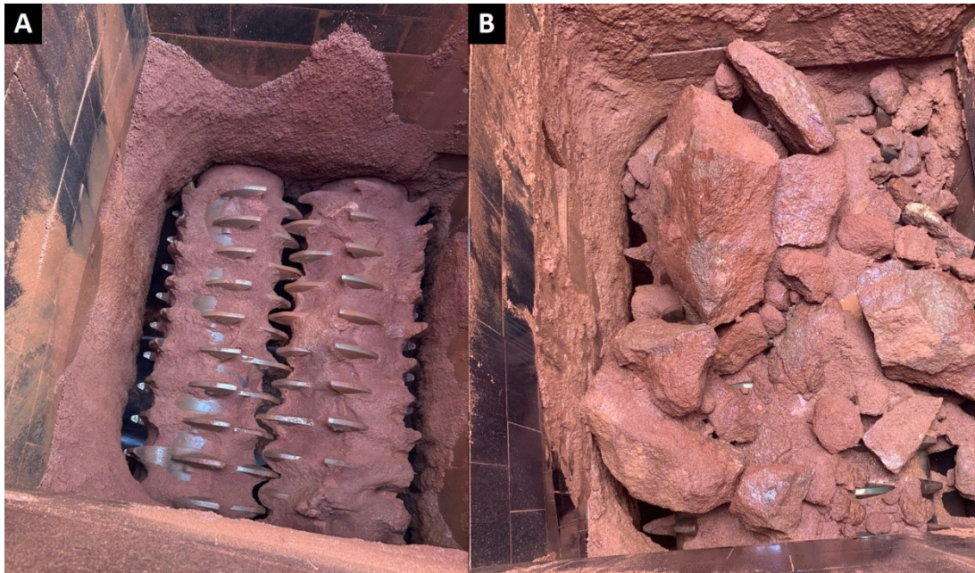
Figure 4. Problematic ore (i.e., A: sticky, B: rocky) in crusher.
